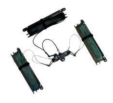
The RF-1941/RF-1940 are lightweight, portable dipole antennas designed for use in the 2 to 30 MHz range with a maximum power of 500 watts. Each antenna is stored on self-contained flat spools with a throwing line to connect to masts, trees, buildings and other structures. The HF antennas can be connected directly to the Falcon® AN/PRC-138, Falcon II® AN/PRC-150 or RF-5800H manpack using the built-in antenna coupler for ALE operation.
