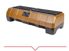
The RF-5857-CH206 is engineered to charge the L3Harris conformal wearable battery (RF-2525/U) for use with Falcon® handheld battery eliminators, power interface adapters and power/data hubs. This six-bay lithium ion solution takes power input from AC and DC sources and includes two USB ports for 5 VDC charging at 2.1A. Battery status is clearly displayed by front panel LED indicator. The RF-5857-CH206 has a small footprint and ergonomic design, ideal for field use and storage.
