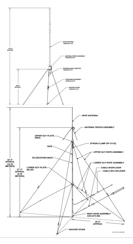
Transportable, Deployable broadband VHF/UHF/L-band, Tripod and Mast mounted antenna systems. Depending on the configuration, it shall be deployable on top of a 27 ft telescoping mast or on the ground standing on its tripod base.
