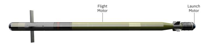
The Raytheon-produced Stinger missile is launched by a small launch motor that pushes it a safe distance from the operator before engaging the main flight motor. L3Harris provides both solid propellant rocket motors.
