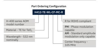
H412-TE-532-105-AM-R is the standard configuration. Please contact L3Harris for additional configurations. Requires H-400 AOM series compatible driver and cable. Specifications subject to change without notice.
