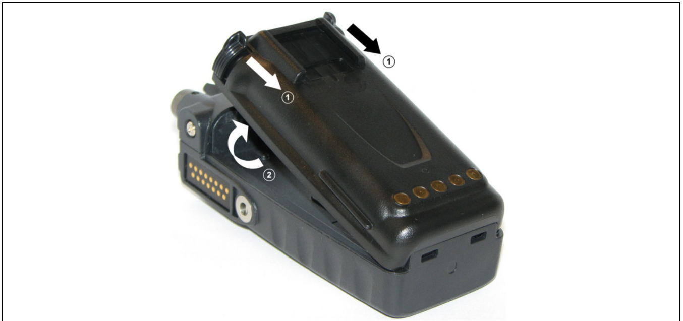
Figure 3-2: Remove the Battery
