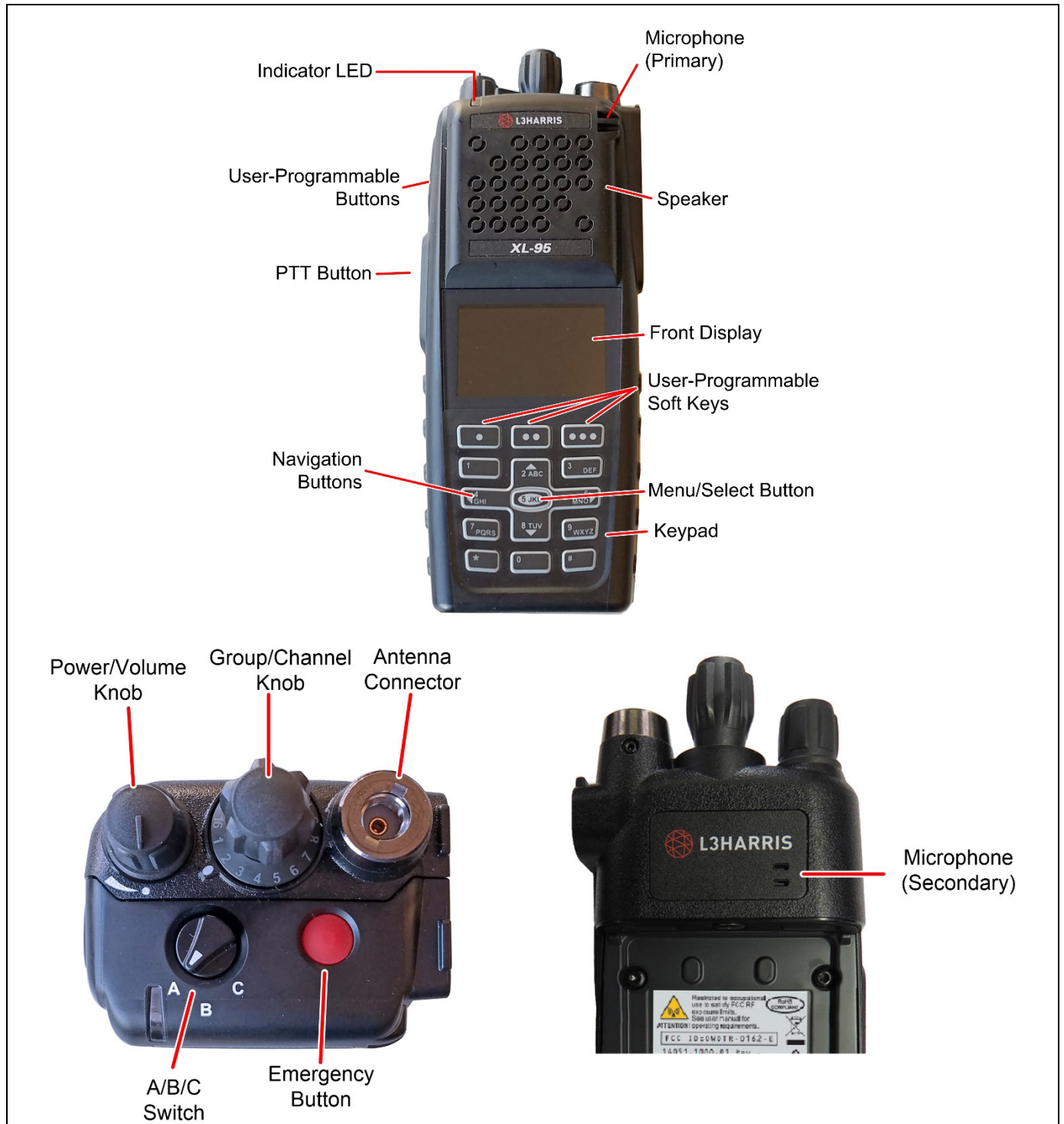
Figure 4-1: Radio Controls, Indicators, and Connectors
