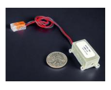
The JAM-11F is an "eye-safe" 1.54 µm diode-pumped passively q-switched Erbium glass laser transmitter with no integrated photodiode.
