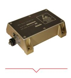
The encrypt and decrypt interfaces are separate, and packets can be simultaneously passed to the AGU for encryption and decryption. This AGU is fully compatible with the Common Communications for Visiting Vehicles protocol used on the International Space Station, as well as other AES-GCM links. A pair of AGUs can be used to secure a channel.
