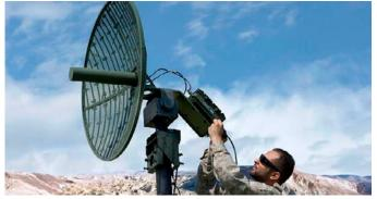
A country wide repeater network extends the range of the RF-7800V/ RF-7850M and RF-7850A network with intelligent retransmission of radio traffic including voice, data, SMS, SA, and directed calling. The system is Scalable and compatible with existing network infrastructure, the solution provides coverage for fast-moving teams to 'roam' across vast areas without losing connectivity.
