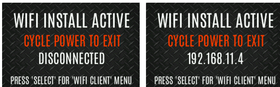
Figure 12-5: Enable Wi-Fi Programming Mode on Radio
